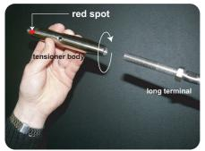
Identify the tensioner body and the long terminal at the other end of the wire. Thread the tensioner (end without the red spot) onto the terminal one (anti-clockwise) turn only.
